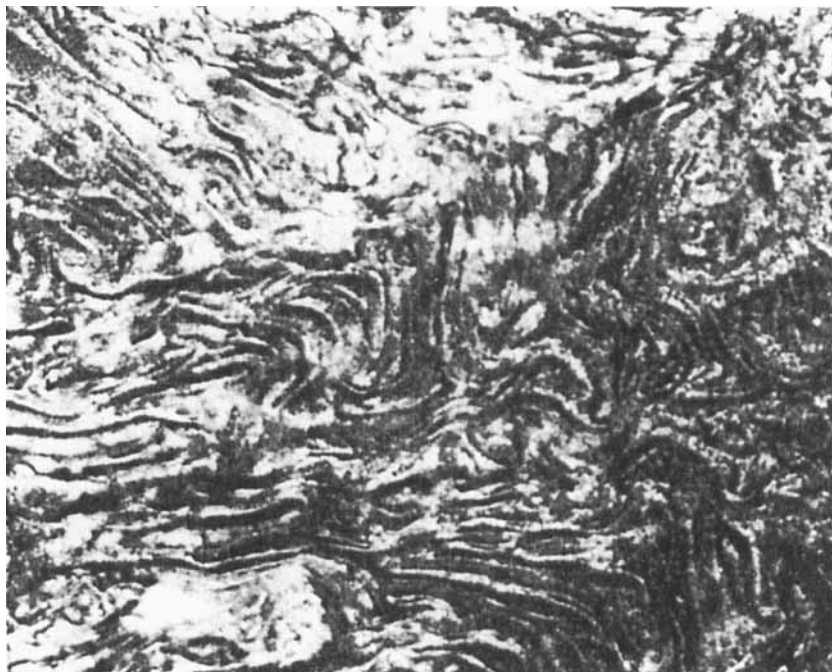
FIGURE 6 Domain pattern retained at 25°C after cooling a 10 \mu\text{m} sample of T2/60 held 4 hrs. at 275°C with 6.4 V.
