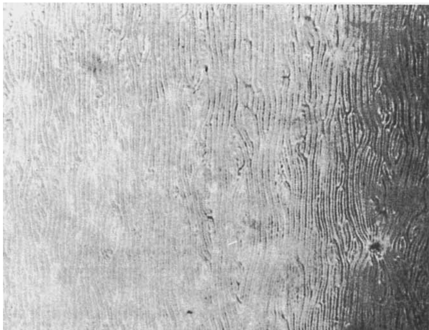
FIGURE 11 VGM pattern observed in a very thin, anchored sample of PAA at 133°C with an a.c. field of 0.05 V and 0.05 Hz (rubbing direction vertical).
