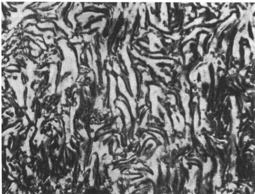
FIGURE 4 Williams domains formed after 6 hrs. in a 10 \mu\text{m} sample of T2/60 at 268°C with 6.4 V. d.c.
