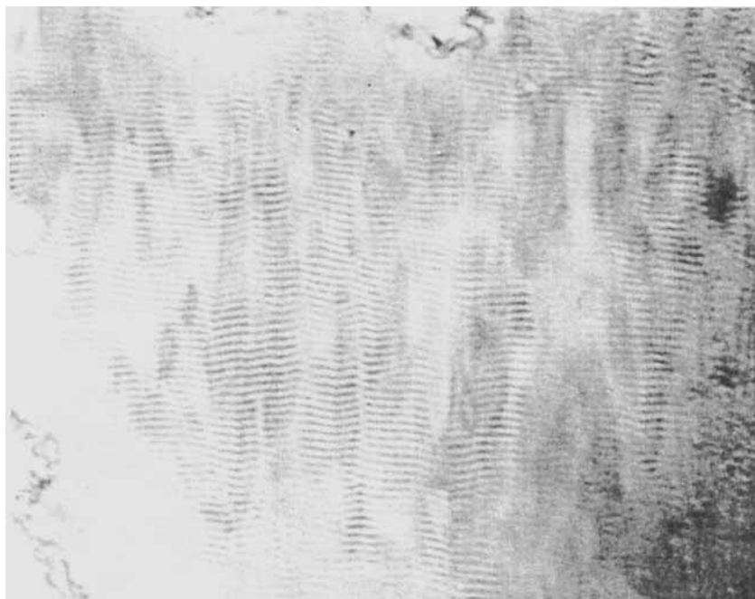
FIGURE 12 Chevron-like pattern formed in the PAA sample of Figure 11 at 19.8 V and 3 kHz (rubbing direction vertical).
